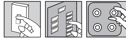
FIG. 1 WALL SWITCH FIG. 2 BREAKER PANEL FIG. 3 FUSE BOX
