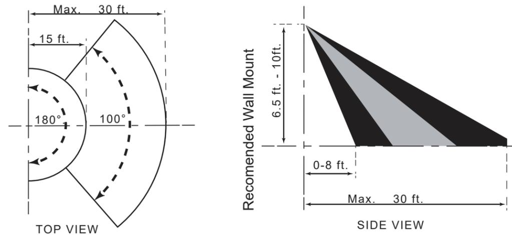
Mount fixture between 6ft.-6in. and 10ft. above the ground. Electrical requirements can be found on fixtures.
