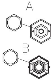
A. When you are installing down, there is a arrow tip on the shade, make sure the arrow face to the wall plate. Fix wall plate into shade like the right picture. Anticlockwise the shade to make sure it was secured and can't move.
